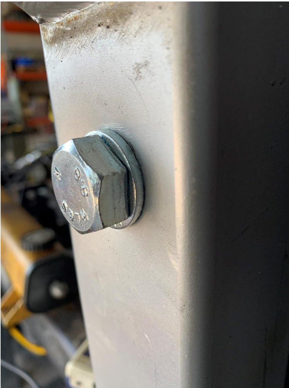
Photograph 2. Detail View of M01 - NBR27-350 Hole deformation during testing.
